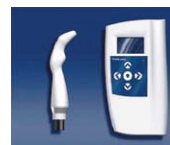
Fig. 2: Ostell Mentor - resonance frequency analysis
