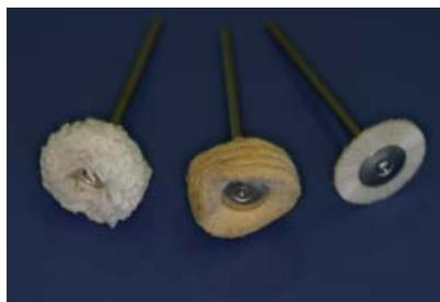
Figure 17: Goat-hair brush and cloth mop for final high polishing in conjunction with diamond polishing paste.
